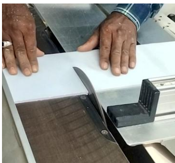
Figure 6: Cutting of acrylic sheets to make nine window panels in a wood cutting machine
