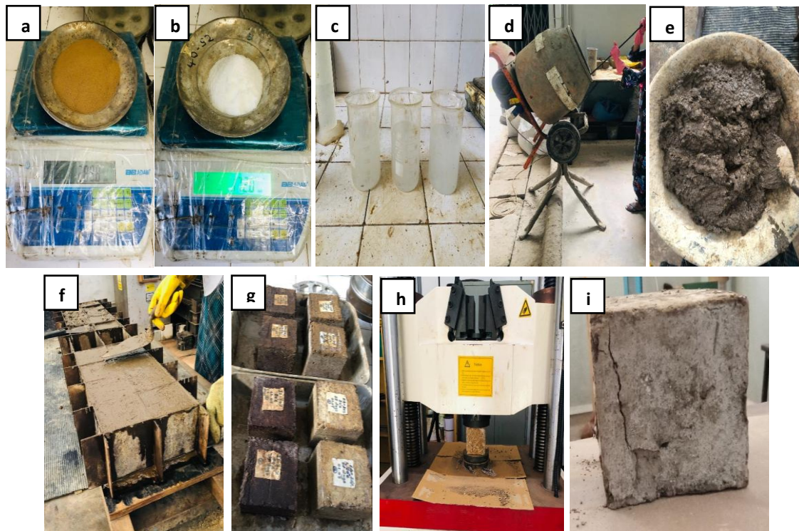
Figure 7: Experimental work (a), (b) measuring materials, (c) preparing NaOH solution, (d), (e) preparing concrete mix, (f) casting test specimens, (g) curing process, (h) testing specimens using UTM, (i) tested specimen
